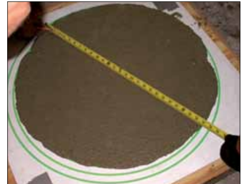
Total spread for SCG should range 22" - 30" (559 - 762 mm) when mixed with the appropriate water content.
