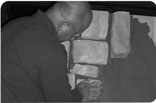
Scott Ellingson/ Twin Cities Concrete Products - Iowa shows the incredible adhesion of the new polymer Modified Stone Veneer Mortar on a test wall for the crowd.
