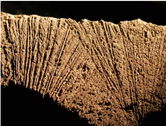
Photo #1: Frozen mortar with frost crystal impression in the typical crow's feet pattern.
