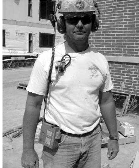
Crew members participating in the SPEC MIX study wear a device that measures exposure to respirable dust and quartz.
