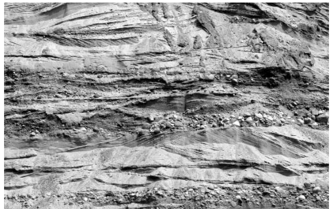
Photo No. 2: Photograph of a glacial outwash deposit. Note the interlayered sand and gravel deposits.
